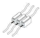
3. Stretch the mounting clip, then put inside the hole carefully.
