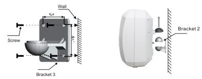
3. According to the installation plan in the adjustable range, adjust the most appropriate height, and then tighten the screws.
